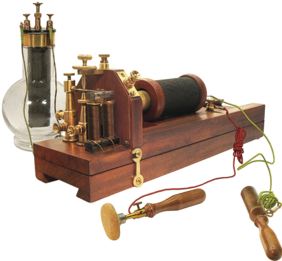
Figure 3. A portable Du Bois-Reymond medical induction device, complete with a Grenet cell and electrodes, very similar to that depicted in André Brouillet's painting (the one in the photo is covered with cotton tissue) Copyright ©Le Compendium/Albert Balasse—2007/2015.
